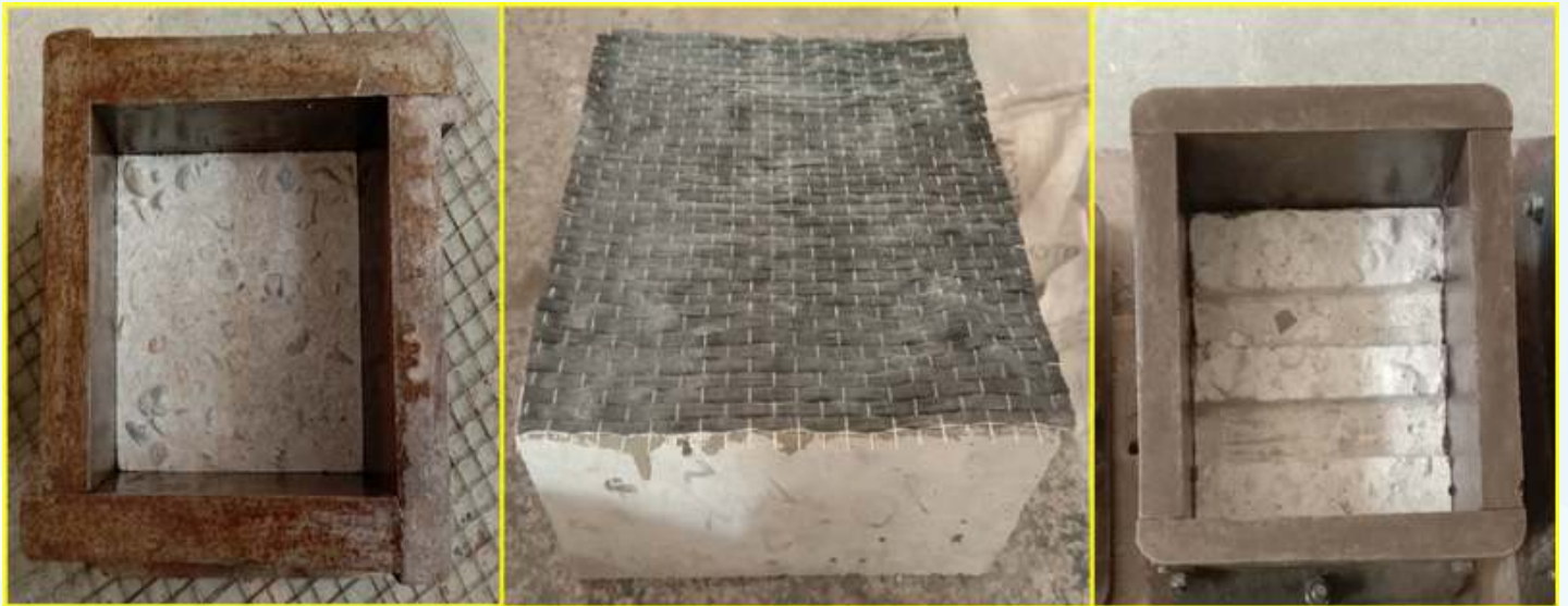
Fig.1 Different surface preparation techniques employed using wire brushing, application of CFRP layer and grooves
