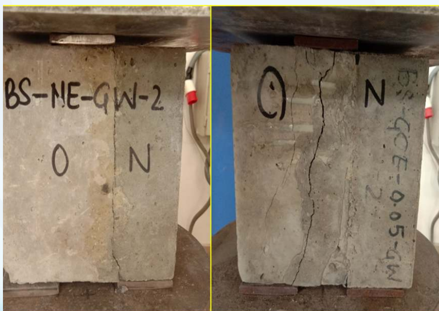
Fig. 2 Failure pattern observed in bisurface shear test with neat epoxy sample on the left and GO-modified epoxy sample on the right under surface preparation technique of wire brushing
